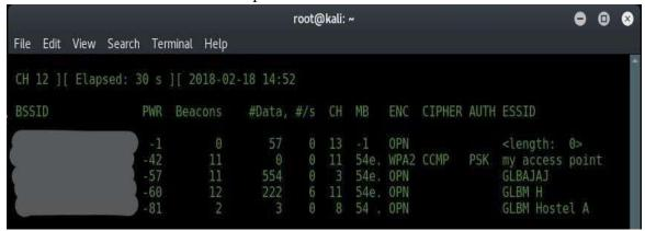
Fig. 5. Scanning of Wi-Fi networks with MAC address and channel
