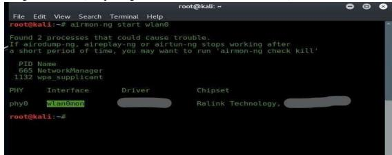
Fig. 4. Enabling monitor mode
