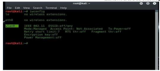
Fig. 3. How to check available interfaces
