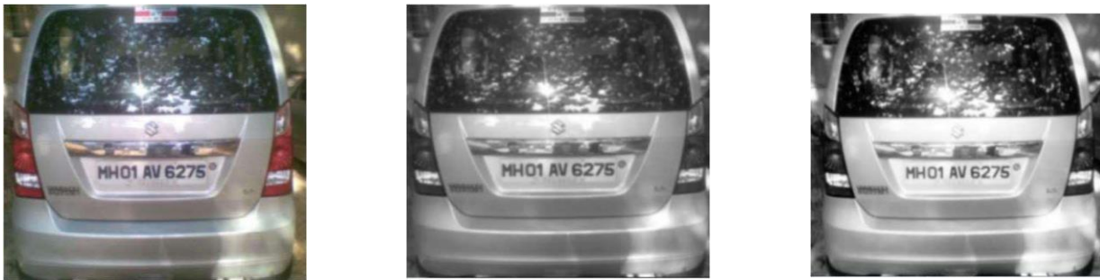
Fig. 2. (a) Loading of image, (b) Gray Scale Conversion, (c) Histogram Equalisation
