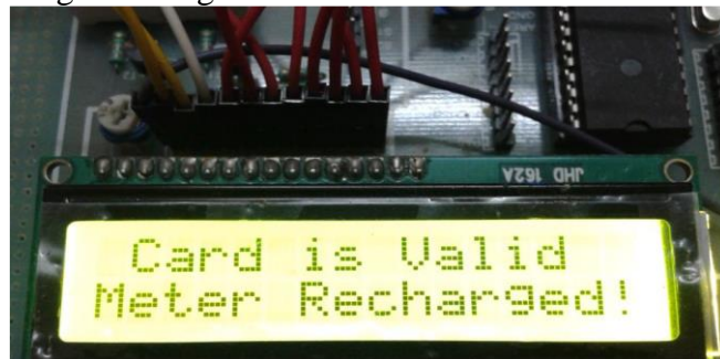
Fig7: Message displayed on LCD screen if card swiped is valid
