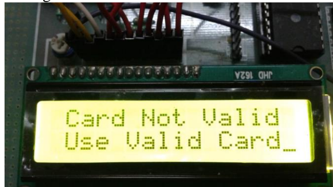
Fig6: Message displayed on LCD screen if card swiped is not valid
