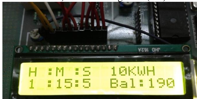
Fig9: Information displayed on LCD screen all the time
