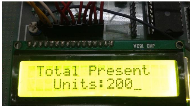
Fig8: Message displayed on LCD screen after meter gets recharged.
