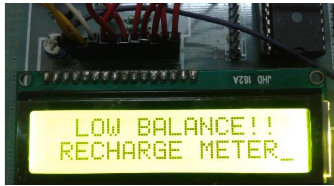
Fig5: Message displayed on LCD screen when meter balance is less than 10 units
