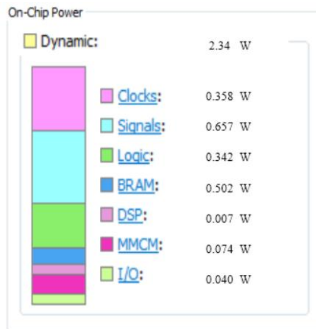
Figure 4. On- Chip Power measurement for HDMI based Video PHY controller at 2 GHz for LVDCI_15 IO Standard
